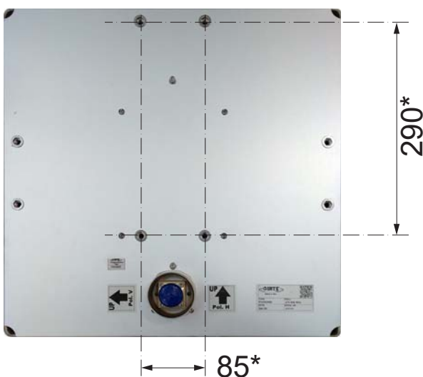
* Fixing Holes for Horizontal Pol. Mount
